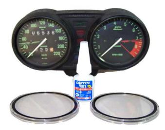
Disassemble the instrument cluster to the point where you have an empty housing. Remove the rubber visors from the front to expose the aluminum rings.
