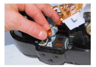
Your new **KATDASH 7880** comes with a "tail" that has the high beam led on the end of it. The end of the "tail" has 2 side flaps, or ears, that are pre-folded and will come packed with a short piece of blue tape holding them folded. Carefully remove the blue tape, and hold the ears folded down as shown. Insert the tail with the ears folded down into the high beam tunnel.
