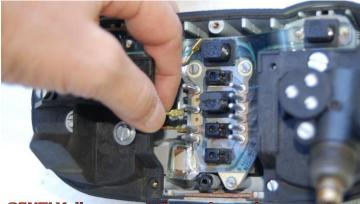
**GENTLY disconnect the tach spade connectors pull on the connector- not the wire!**
