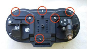
remove 6 screws in "T" shaped rear cover
