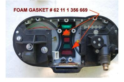
After you remove the old bulb carrier, make sure you have the foam gasket that should be against the lens face. p/n 62 11 1 356 669. This gasket keeps the each light's glow from seeping out of its own lens compartment, or the white gauge light from leaking in. If yours is missing or damaged, they are available from Max BMW or Bob's BMW online. to install outer O-ring gasket remove 3 screws each side holding the instruments in
