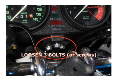
Remove your instrument pod from your motorcycle. First disconnect the speedometer cable from the back. Then loosen the 3 bolts or screws that hold the pod on the mounting bracket. It is not necessary to remove these bolts. After you loosen the bolts the pod should slide up off of the bracket.
