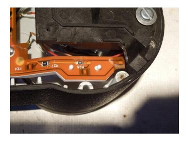
Make sure that the flexible circuit board is tucked in at the end of the arms, and not caught on the instrument back on either side.
