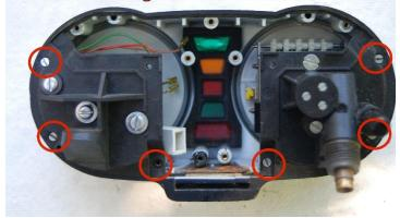
If you are going to replace the outer 'O'-ring gasket- now is the time to do that. Remove the 6 screws that mount the tach and speedo to the case. Refer to the gasket install instructions (available on our website) for further directions and photos.
