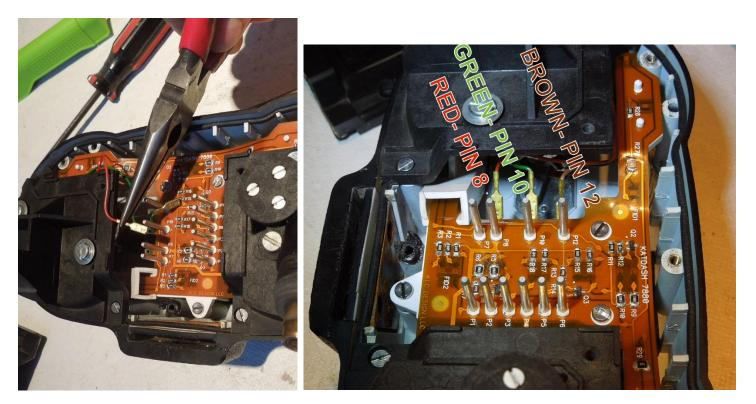
Using a needle-nose plyers, reconnect the tach wires. Be sure to hold the connector by the metal crimp collar. The RED connector goes to Pin 8. The GREEN connector goes to Pin 10. The BROWN connector goes to Pin 12. (FYI- the pin numbers are marked on the new flex.)
