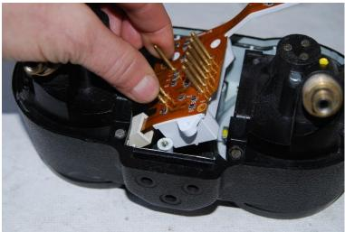
Slide the rest of the tail into the tunnel as you insert the main unit into the center of your instrument pod. It will drop right down onto the original mounting posts. Check that the end of the arms flex is clear- see next photo.
