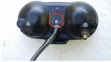
Now that you are able to move the pod a little, you have some access to the rear plug. There is a small phillips screw in the middle of it. Remove this screw, and **gently** wiggle the plug loose. Often the plug joints are jammed with dirt and crud. And sometimes there is corrosion inside the plug itself. Be gentle and patient- this plug is also NLA.
