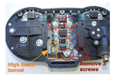
Remove the 3 screws that hold the oem bulb carrier in, and remove the bulb carrier.
