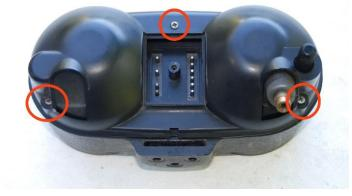
Remove the 3 screws that hold the outer cover on.
