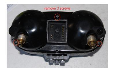
Remove the 3 screws that hold the outer cover on.
