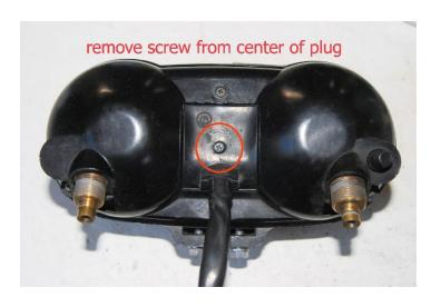
Now that you are able to move the pod a little, you have some access to the rear plug. There is a phillips screw in the middle of it. Remove this screw, and *gently* wiggle the plug loose. Often the plug joints are jammed with dirt and crud. And sometimes there is corrosion inside the plug itself. Be gentle and patient- this plug is also NLA.
