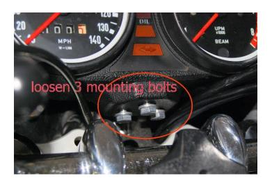
Remove your instrument pod from your motorcycle. First disconnect the tach and speedometer cables from the back. Then loosen the 3 bolts that hold the pod on the mounting bracket. It is not necessary to remove these bolts. After you loosen the bolts the pod should slide up off of the bracket.
