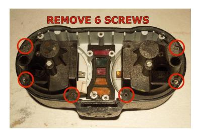
If you are going to replace the outer 'O'-ring gasket at this time- now is the time to do that. Remove the 6 screws that mount the tach and speedo to the case: 3 per side. Refer to the gasket install instructions (available online on the FAQ page) for further directions and photos of the O-ring installation.
