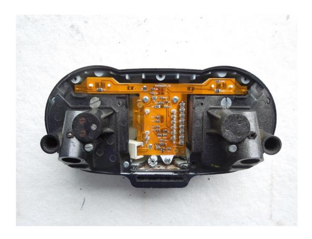
Re-install the 3 screws from the original bulb carrier in the new KATDASH unit. Here it is correctly installed.
