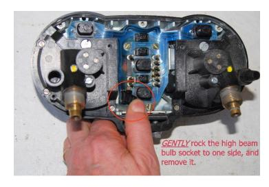
Now the oem bulb carrier is accessible. Before you can remove it, you have to take out the high beam bulb socket at the lower left side. To remove any bulb socket, you rock/tip it to one side until the spring contact pops out. (see above) Be very gentle, the copper flaps/ears are old and fragile. This is one of the basic problems with the original bulb carriers as you probably already know.
