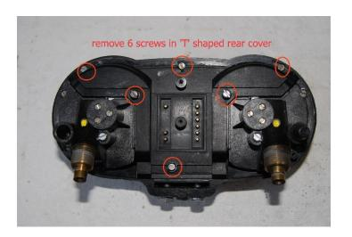
Remove the 6 screws that hold the rear 'T' shaped cover on. Note: the 2 screws at the corners of the gauges are not machine screws like the others. Keep track of which screw goes where.
