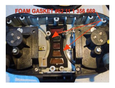
After you remove the old bulb carrier, make sure you have the foam gasket that should be against the lens face. p/n 62 11 1 356 669. This gasket keeps the each light's glow from seeping out of it's own lens compartment. If yours is missing or damaged, they are available from Max BMW or Bob's BMW online.
