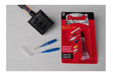
Now is a good time to clean and put some contact cleaner in the terminals of your old plug. I like to use one of the dental pick/brushes and some DeoxIT D-5. DeoxIT will improve electrical contact between the plug and the light unit, as well as help prevent oxidation in the future. But any quality contact cleaner and lubricant will do. I sell a DeoxIT kit with brushes on the website.
