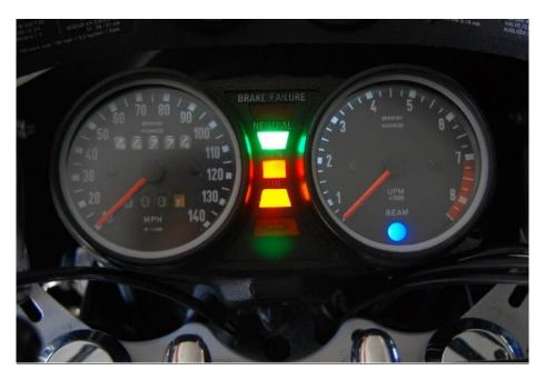
Here is a photo with the KATDASH /6 installed and the ignition key on. (the bike is not running, & in a dark garage ) Your Neutral, GEN, and OIL lights will light up. The brake failure light does **NOT** light up unless there is a failure in the system. You can test your brake failure light by removing your gas tank, and shorting across the 2 terminals on the master cylinder reservoir cap.
