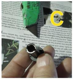
You will need to file, or trim (with a utility knife) off the top plastic rim of the insulated socket, to get the led bulb to insert deep enough in the bulb socket.
