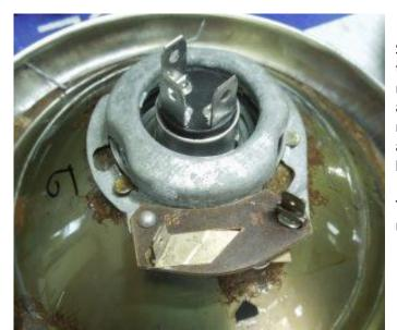
So far, I have seen 3 different parking light bulb assemblies: the stock/original headlight bulb collar (left) which is spring mounted on 3 tabs. The Parking light is under the bakelite assembly (bottom of photo) and sticks down through a round hole in the reflector. If this is what your headlight assembly looks like: YOU WILL NEED TO MODIFY IT to get the led bulb installed. Details below.
