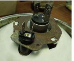
Another assembly we found was a modified original bulb collar with the original parking light assembly removed, and a stock BA9 insulated socket installed. (photo left)
