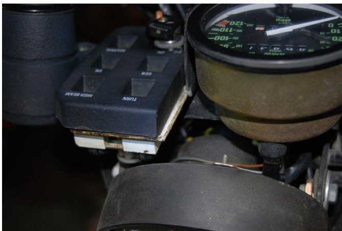
Unplug the telltale electrical connector- the white circular plug.
