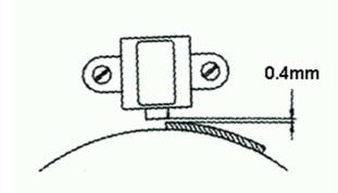
Now, again turn the rotor by hand and check the gap between the sensor and the rotor's elevation. It has to be 0.4 (max 0.5) mm. Adjust it by loosening the sensor's mounting screws and shifting the sensor a little. Do not forget to fasten the screws well after that.
