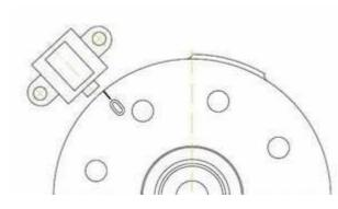
Than place the rotor back onto the shaft in such a way, that the 0-marking line aligns with the rh edge of the sensor pin as shown in the sketch here.
