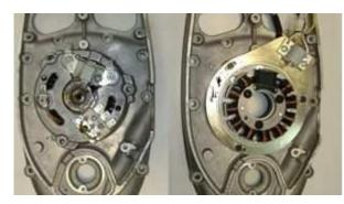
Put the pre-assembled stator plate instead of the original alternator onto the engine case.
