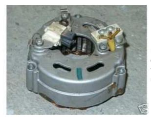
Disconnect all cables at the alternator, condenser, points (or hall element), ignition coils, the diode plate and the regulator unit and remove those parts.
