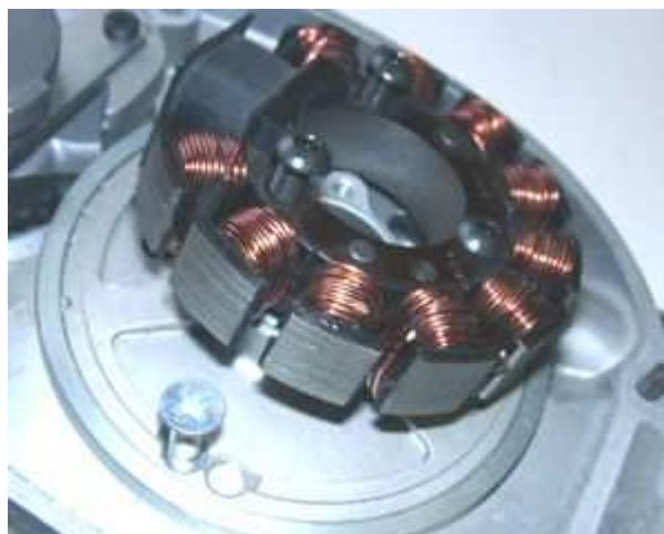
The new stator unit is pre-assembled so that you can recognize its structure more easily. To install it, it has to be partially disassembled however. Take care not to damage the paint insulation of the coils.
