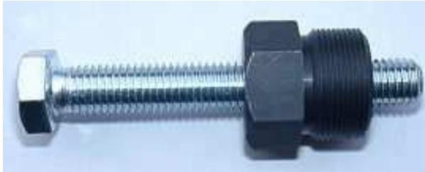
To disengage your new rotor again, you will need a puller M27x1.25 (part-no.: 99 99 799 00 -**Not provided!**-).
