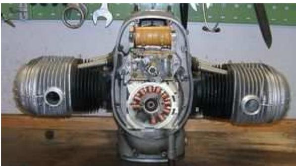
Now put the stator coil back into its position on the plate, taking care not to damage the wires. Make sure that the inner opening of the stator unit slots evenly over the elevated fixing rim of the base plate - otherwise the coil will sit loopsided and will touch the rotor, damaging it.
