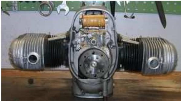
Put the rotor onto the crank and screw it down with the provided screw M8x40. Do not forget to place the washer there.. To disengage the rotor again, use a [puller M27x1.25](#), never a claw puller or hammer blows!
