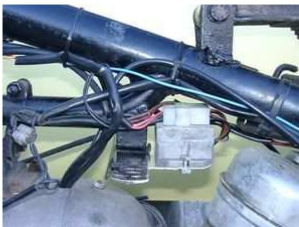
The new regulator/rectifier could be fitted under the rear holder for the petrol tank. (On this proposal the customer has used a selfmade [unit plate](#).) For this, unscrew the nut (spanner 13) securing your BMW's tank holder and put your new regulator plate (with the regulator on it) underneath. The regulators cooling fins will face upwards. Put the nut back, do not forget to put the washer back.
