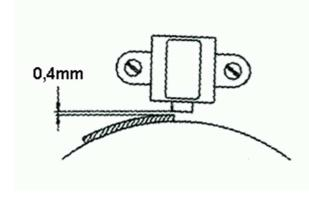
Turn the new rotor by hand and check the gap between the pick up and the elevated nose (protrusion) on the circumference of the rotor. This has be be set to 0.5mm. You may set the gap by loosening the 2 holder screws a little and shifting the unit accordingly. After setting the gap, make sure to fasten to 2 screws properly. Even if by chance the gap was correct, fasten the screws! They are loose at time of delivery.
