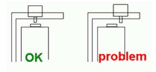
With the rotor set, check that the protrusion runs in level with the the sensor and not outside its track
