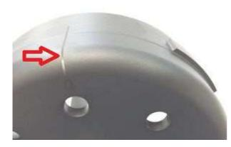
Have a look at the new rotor. You will find on the circumference some long protrusion and a lasered on line which goes right up to the top where it is marked with a "0".
