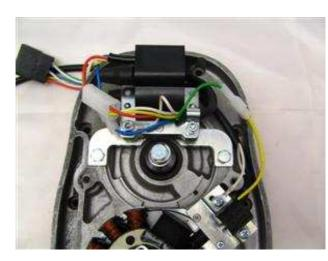
Screw the 2 high tension cables (if supplied as one, cut it into 2) into the ignition coil.
