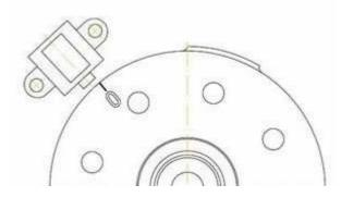
Than place the rotor back onto the shaft in such a way, that the 0-marking line aligns with the rh edge of the sensor pin as shown in the sketch here.
