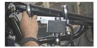
The new electronic advance unit is premounted on a holder plate which itself will be fitted with 3 clamps to the frame under the petrol (gas) tank.
