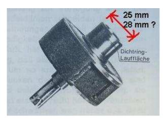
Check the diameter of the sealing stud on the original magneto rotor. You normally have here 25mm. On R68 and some R69 however that is 28mm.
