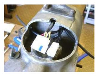
The short harness pieces running from the new generator und the coil unit will be ushered with theirs plug-ends through the top opening into the rear top engine compartment. They wait there to get connected to the rest of the assembly.
