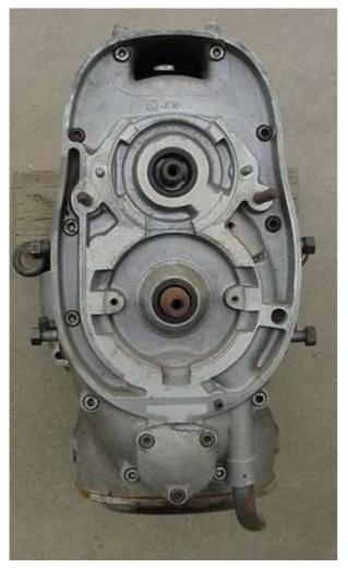
Use a hex key 6mm and remove the screw that retains the advance unit and the magnetic rotor on the nose of the camshaft. To do that, you will have to hold the generators rotor with your hand using a piece of cloth to avoid injury. Take the centrifugal advance unit off.
