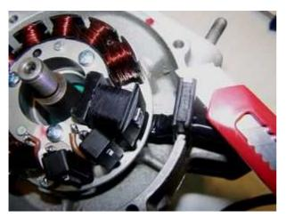
There is a rubber grommet on the stator wire. Press it into the wire exit opening and than cut the surplus material off carefully.
