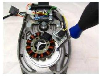
The new stator unit is pre-assembled so that you can recognize its structure more easily. To install it, it has to be partially disassembled however. Take care not to damage the paint insulation of the coils. Unscrew the new stator coil from its base plate (the 3 hex screws) and lift it a little away from it so that you can access the mounting holes in the base plate.
