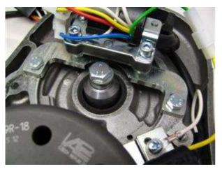
Place the provided oil-seal cam onto the camshaft and fasten it with the special screw M8x40. Please don't forget to use the provided washer.
