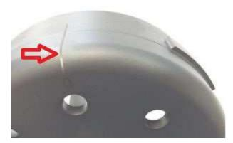
Have a look at the new rotor. You will find on the circumference some long protrusion and a lasered on line which goes right up to the top where it is marked with a "0".
