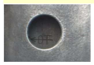
Take the spark plugs out. Place the rotor provisionally onto the crank shaft (without screwing it down there) for using it as a turning knob. Bring the crank shaft into TDC (in German OT) by using the spyhole.
