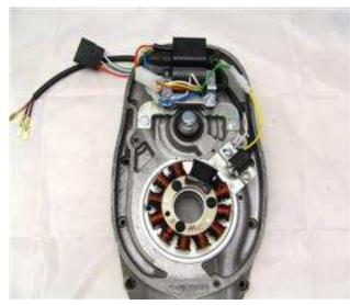
Now put the stator coil back into its position on the plate, taking care not the damage the wires. Make sure that the inner opening of the stator unit slots evenly over the elevated fixing rim of the base plate - otherwise the coil will sit loop sided and will touch the rotor, damaging it.
