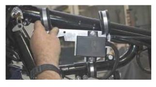
The new electronic advance unit is premounted on a holder plate which itself will be fitted with 3 clamps to the frame under the petrol (gas) tank.
