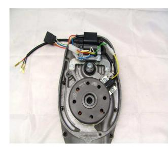
Magneto with integrated solid state ignition, output at 12V/150W DC. Ignition with own power supply from within the system. Replaces old generator <u>L45/60L</u>, regulator, magnet unit, centrifugal advance unit in above listed BMW with either 17 or 20mm crankpin (measured at wide end).
