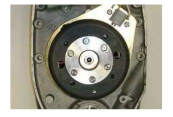
Place the rotor onto the crankshaft and fasten it with the screw M8. Do not forget to place the washer underneath.
