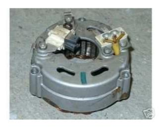
Disconnect all cables on alternator, diode block and regulator and remove those parts.
