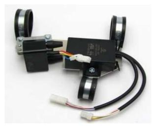
Mount the electronic regulator/rectifier, the advance unit, the ignition coils and the relay at a convenient place, maybe with a little holding plate (not enclosed) at the frame underneath the tank.
