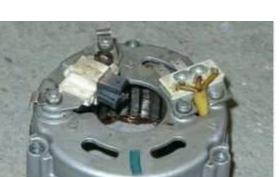
Disconnect all cables at the alternator, condenser, points (or hall element), ignition coils, the diode plate and the regulator unit and remove those parts.
