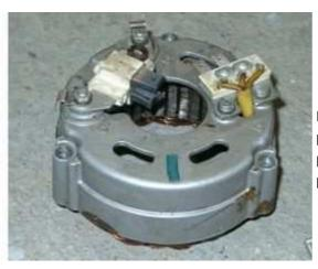
Disconnect all cables at the alternator, condenser, points (or hall element), ignition coils, the diode plate and the regulator unit and remove those parts.
