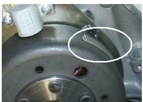
Have a look at the new rotor. You will find on the circumference some long protrusion. This is to trigger ignition. However it does not do so when this elevation reaches the sensor, but after it has gone past it as the system needs to calculate the advance based on engine speed (the time the protrusion needs for one passage used as reference).
