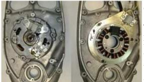
Put the pre-assembled stator plate instead of the original alternator onto the engine case.
