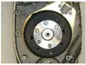
Take the spark plugs out. Place the rotor onto the crank shaft (without screwing it down there) for using it as a turning knob. Bring the crank shaft into FZ position (maximal advance) by using the spyhole.
