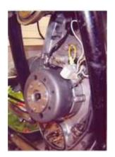
Magnet based generator with integrated solid state ignition. Output 12V/190W DC. Maintenance free, electronic ignition with own power supply from within the system. Replaces the stock 12V alternator (including diode plate and regulator) as well as all ignition parts, be it points or hall element). There is no need for changes on engine casing.
