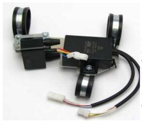
Mount the electronic regulator/rectifier, the advance unit, the ignition coils and the relay at a convenient place, maybe with a little holding plate (not enclosed) at the frame underneath the tank.
