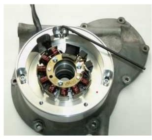
Place the pre-assembled new generator unit onto the engine.
