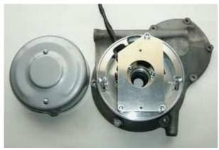
Once all is done and engine runs to your satisfaction, place the cover holder plate back. Under the plate come again the 3 spacer tubes. 3 screws M6xc30 fasten all.
