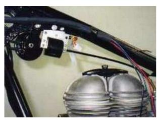
Fasten the new ignition coil beneath the petrol tank or on the frame.
