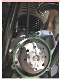
Magnet based generator with integrated solid state ignition. Output at 12V/180W DC. Ignition with own power supply from within the system.
