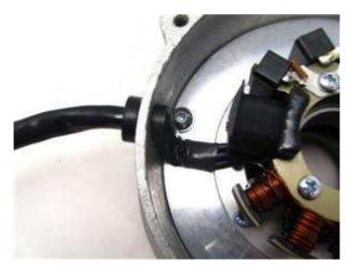
Pull the enclosed grommet over the cable and push it into the engine opening (a drop of oil will help).
