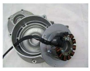
Lead the stator harness from the inside through the cable hole at the engine.
