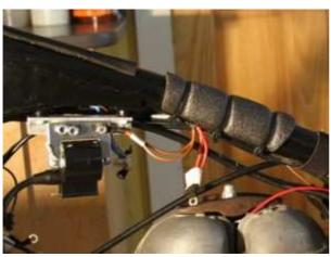
Fasten the new ignition coil beneath the tank. At some chassis is there a holder lug. If not, you can help yourself with <u>a selfmade bracket</u> or wire binders.
