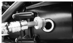
2. Ensure that the old seal ring came off with the original plug. Screw in the Oil-Eye with the supplied seal ring.
