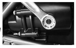
The transmission oil level should be at the bottom of the hole, so the oil level may not be visible through the OilEye when the bike is upright. In most cases, it will be necessary to tip the bike to the side to see the oil level. Be very careful when doing this, that you do not drop the bike. It's best to have a friend tip the bike or spot the oil level for you!
