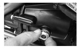
3. Tighten the OilEye with a 22mm wrench or socket. (Tip a 7/8" tool will also work.
