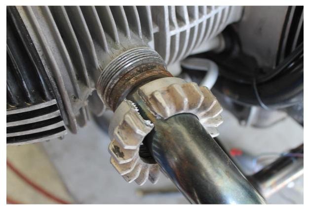
If the threads are damaged, in many cases they can be repaired with a thread file or better yet, a cutting die. These tools are available on <a href="http://www.boxer2valve.com">www.boxer2valve.com</a> and also <a href="http://www.wunderlichamerica.com">www.boxer2valve.com</a> and also
