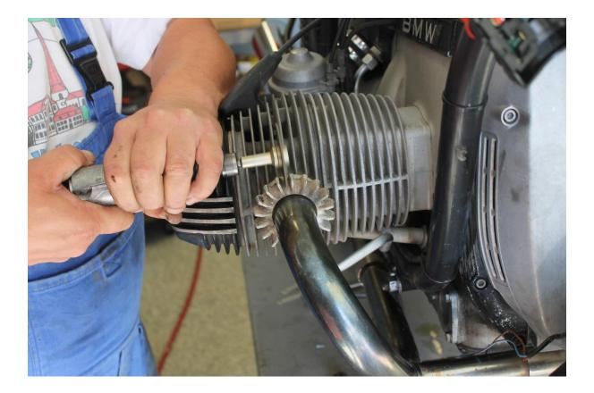
Once you have cracked through the nut, spread it apart. You can use a screwdriver to pry between the fins of the nut. You can also use some suitable pliers. I have some old piston ring pliers that work great for this as you can see in the picture below.
